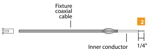
3 Slide slotted flared end Strain Relief down coaxial cable.
