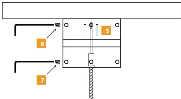
6 Once the Coaxial cable stops, tighten set screw snuggly.
